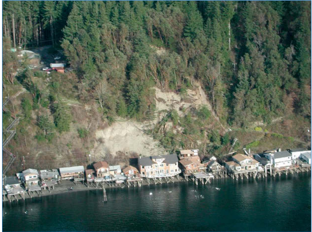
Figure 2-9: Aerial view of Salmon Beach landslide caused by the 2001 Nisqually earthquake.
